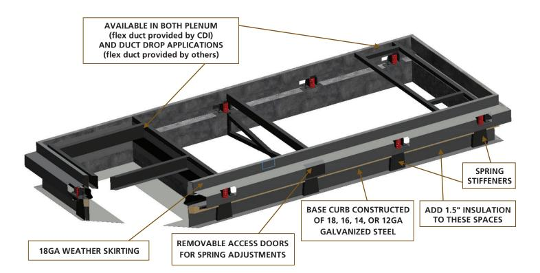
6. Remove the spring access panels and follow the instructions below to adjust the springs.
