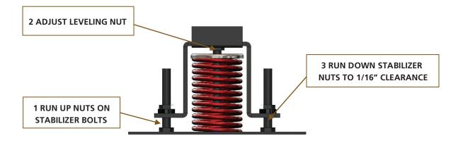
These high quality isolators are equipped with stabilizer bolts and leveling nuts which must be properly adjusted to provide full isolation. They may be bolted to any mounting surface that is within <sup>1</sup>/<sub>4</sub>" of being flat & level. After positioning the equipment squarely on the isolators, use the following adjustment procedure.
